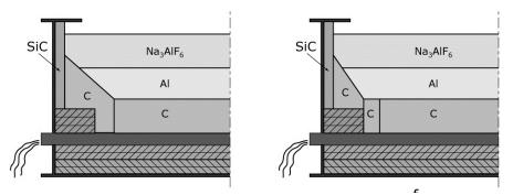
Figure 1. Different zones in SiC side lining.
